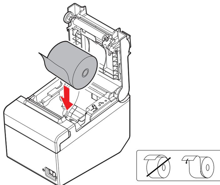
3. Pull out some paper, and close the roll paper cover. When the printer power is on, the roll paper is automatically cut.
