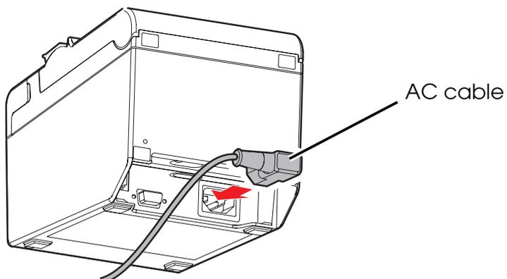
5. Insert the AC plug into a socket.
